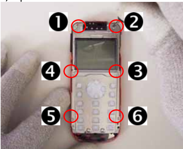
7) Remove the six #5 TORX screws in the order shown.
